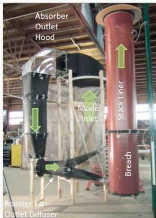
Figure 4: Detailed scale model of the FGD plant, outlet duct and chimney breeching to develop, test and validate the proposed liquid collector and drain system.
