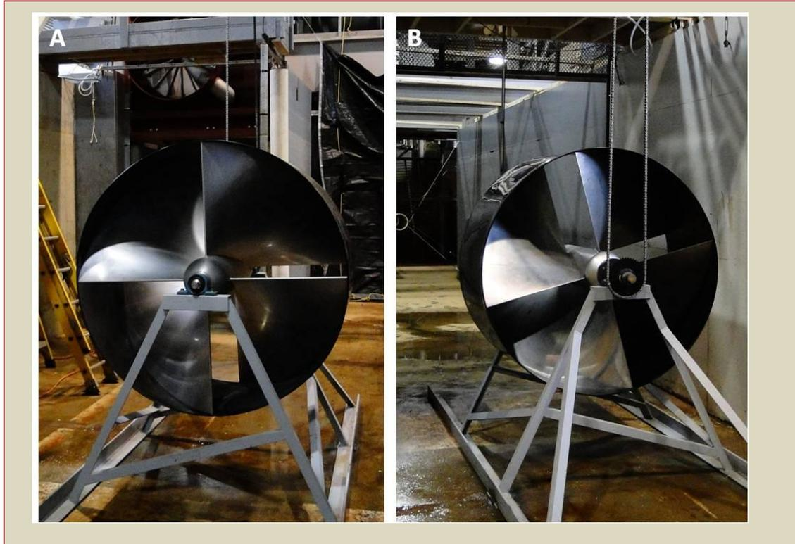
Figure 2. Downstream (A) and upstream (B) views of the Welka UPG turbine installed in Alden's large flume test facility.
