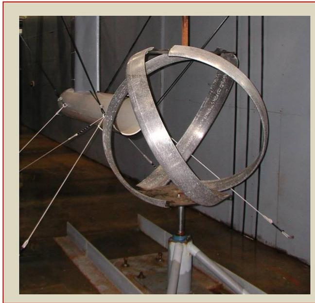
Figure 1. The Lucid Spherical Turbine (LST) installed in Alden's large flume test facility (looking upstream with fish release tube in background).
