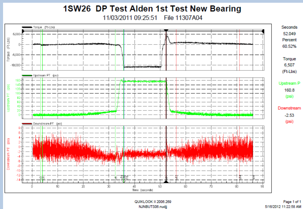
Figure 1: Traces of torque, upstream pressure and downstream pressure (a) before the installation of Bal-Seals and (b) after the installation of Bal-Seals.
