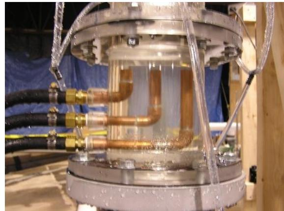
**Figure 6** Isokinetic sampling section downstream of strainer module.
