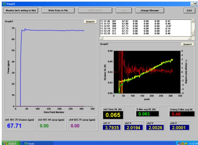
**Figure 7** Data acquisition screen view of instantaneous test results, including flow rate (blue), instantaneous total pressure head loss (yellow), five minute averaged head loss (green), and percent change in head loss over a five minute period (red).
