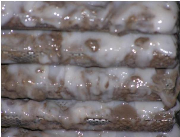
**Figure 9** Side view of a strainer after head loss testing.
