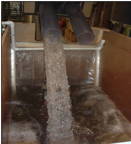
Fish Return System Testing Facility - 2 ft Drop
