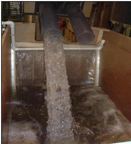
Fish Return System Testing Facility - 2 ft Drop
